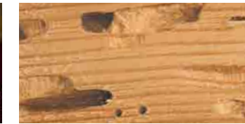
· DAMAGE Exit hole: oval > 2 mm Bore dust: coloured cylinder Timber attacked: sapwood of softwoods
